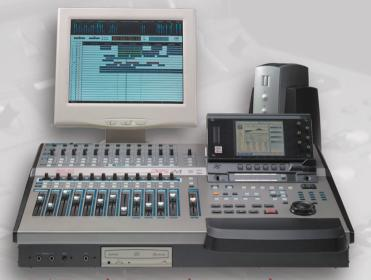
24 Tracks of uncompressed 16/24-Bit recording and playback at 32/44.1/48/88.2 and 96kHz for absolute audio quality and a 44-channel automated digital mixer with professional, long throw (100mm) touch sensitive motorized faders. With the Q-Strip, The trip, the Q-Channel and the six Q-Link encoders you're in total charge of the machine. Never before has such a tactile user interface been offered on a digital personal studio.
